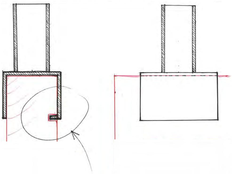
The sketch shows the metallic fasteners bent around the wooden frame and kept in place through a small tenon that fits into a spring.
