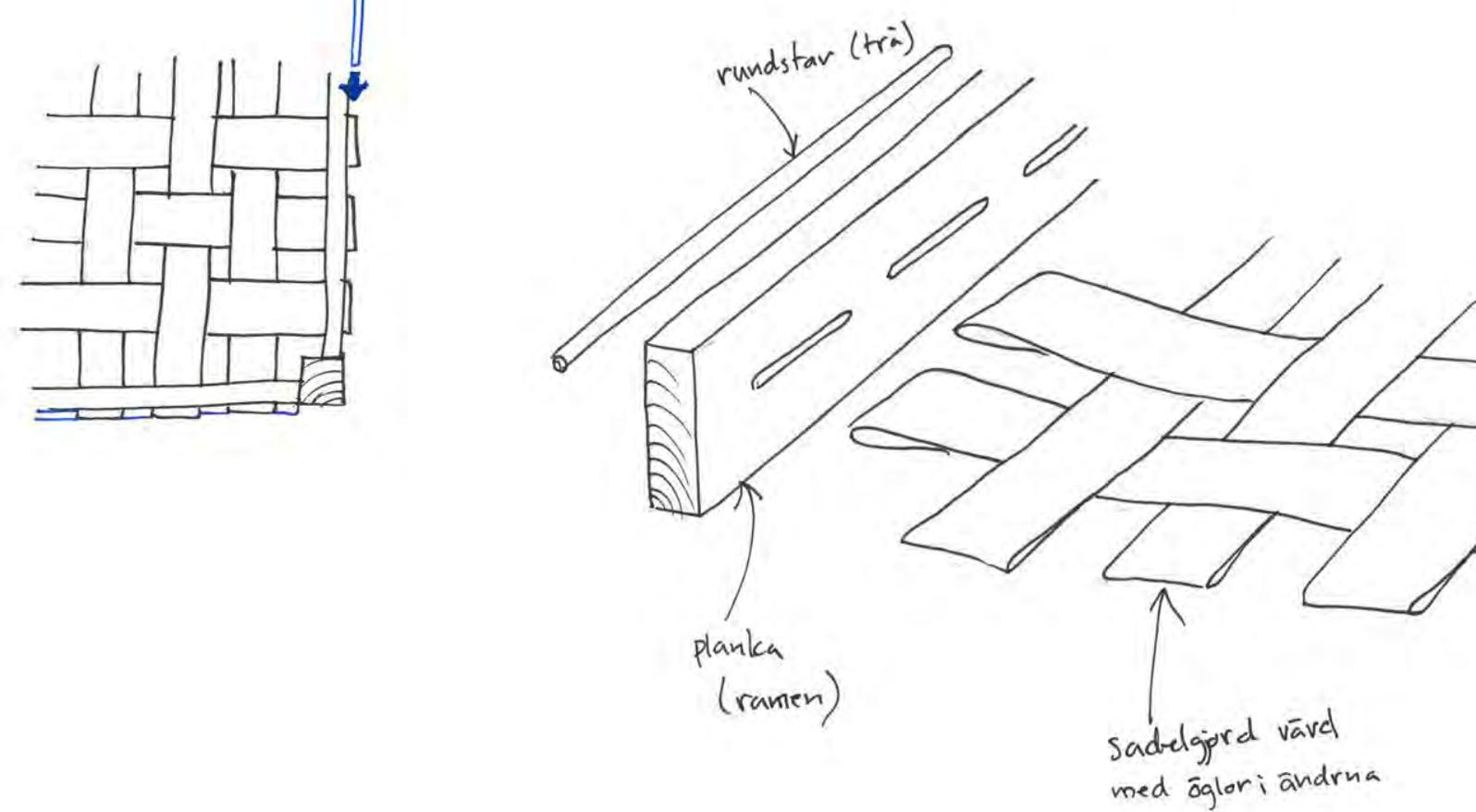
The braided saddle girth mesh has loops at the ends, these are placed through slots in the frame, a stick goes through on the other side and holds it in place.
