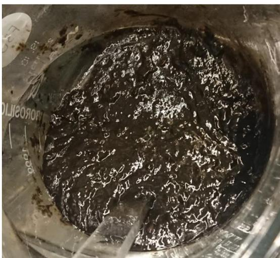
Figure 10. Textiles dissolved in 80% sulfuric acid.
